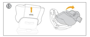
13 - Pull the softgoods up around the seat shell and completely remove.
