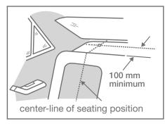
If drilling a new hole, select a position on the centre line of the seating position, and no closer than 100 mm from the front edge of the parcel shelf.
