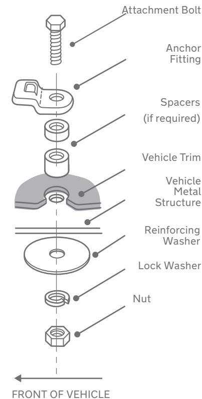
If drilling a new hole, select a position on the centre line of the seating position, and no closer than 100 mm from the front edge of the parcel shelf.
