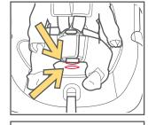
IMPORTANT: After changing the strap position pull firmly upward on the crotch strap to check the buckle is securely fitted.
