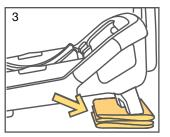
IMPORTANT: Any extra padding placed under the base must be firmly folded so that when the vehicle belts are pulled up tight, the base is secure.
