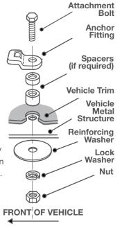
For vehicles other than sedans - In Australia, consult your nearest child restraint fitting station or traffic authority for vehicle inspection to find the best, correct position for the placement of the anchorage point, and for the correct at-tachment bolt length and use of spacers. In New Zealand, consult the agent for the vehicle.
