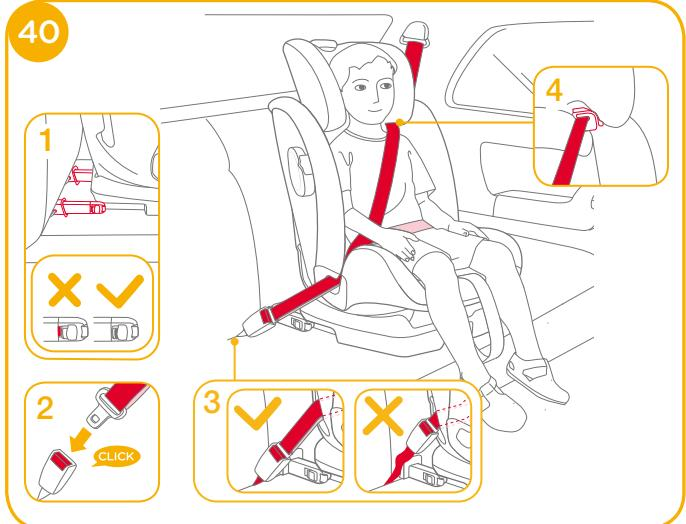
1. Make sure that both Isosafe connectors are securely attached to their ISOFIX anchor points. The colors of the indicators on both Isosafe connectors should be completely green. 40-1
