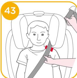
To ensure the correct head support height is obtained, the bottom of the headrest MUST be even with the top of child's shoulders as shown in ④2 and the shoulder belt must be positioned in the red zone as shown in ④3.
