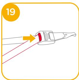
2. Connect the tether hook securely to the anchorage fitting. 20
