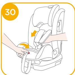
2. Press the red button to disengage the buckle. 31
