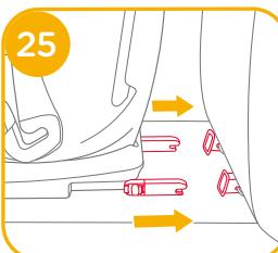
! Make sure that both Isosafe connectors are securely attached to their ISOFIX anchor points. The colors of the indicators on both Isosafe connectors should be completely green. 26
