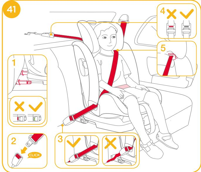
1. Make sure that both Isosafe connectors are securely attached to their ISOFIX anchor points. The colors of the indicators on both connectors should be completely green. 41-1
