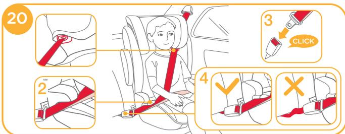
! Could also be installed by using 3-point belt only. (see images [20](#) - [24](#))
