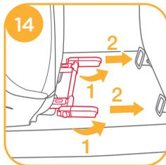
4. Line up the Isosafe connectors with the ISOFIX anchor points, and then click both Isosafe connectors into the ISOFIX anchor points. **15**
